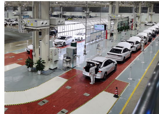
Fitting-out Inspection Line at GAC AION's Intelligent Ecological Plant
